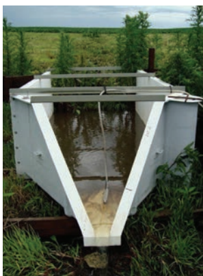
These flumes measure surface water runoff from the STRIPS watersheds. Note the amount of sediment displaced from a 100 percent no-till crop field (left) compared to a field enhanced with 10 percent prairie (center) and a field of 100 percent prairie, which has little sediment loss.
