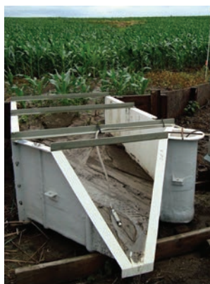
These flumes measure surface water runoff from the STRIPS watersheds. Note the amount of sediment displaced from a 100 percent no-till crop field (left) compared to a field enhanced with 10 percent prairie (center) and a field of 100 percent prairie, which has little sediment loss.
