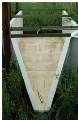
These flumes measure surface water runoff from the STRIPS watersheds. Note the amount of sediment displaced from a 100 percent no-till crop field (left) compared to a field enhanced with 10 percent prairie (center) and a field of 100 percent prairie, which has little sediment loss.
