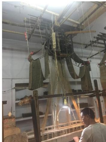
Jacquard looms have a chain of punched cards corresponding to rows in the fabric design. Their use of replaceable cards to control a sequence of operations is considered an important step in the history of computing hardware. "Never thought I would see one in action," said Doug. Here are Doug and Helena in front of the Taj Mahal:
