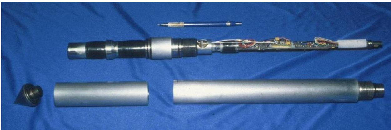
Figure 2. Disassembled cone penetrometer (Saftner and Hryciw, 2015).
