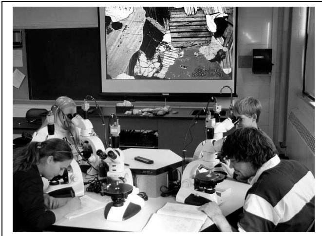
*The new lab includes 15 high-quality binocular student microscopes equipped with some of the best optics available, a research-quality microscope for instruction and student projects, a digital imaging system, a computer for acquisition and processing of images, a video system to network all of the student scopes to a live display, dual video projectors, and new furnishings for the work areas.*
